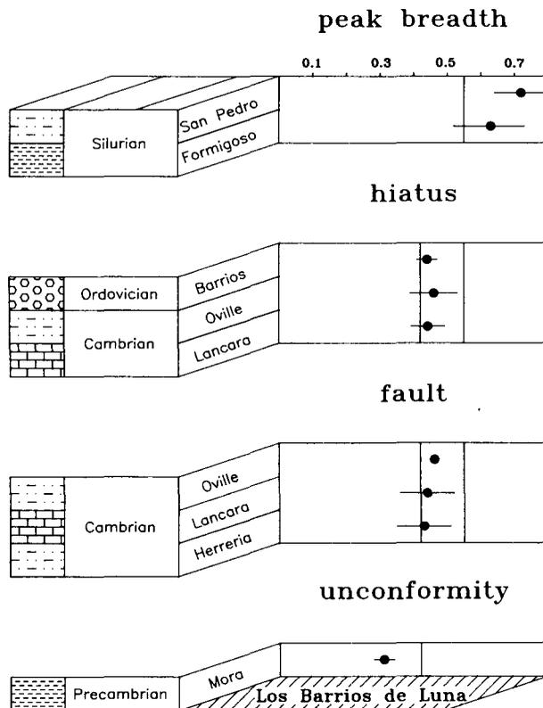
Fig. 3.—Distribution of IC in the section near Los Barrios de Luna (transect G in fig. 5): The average of all samples of each formation demonstrates the jumps at the Precambrian/Cambrian and Cambro-Ordovician/Siluro-Devonian contacts as well as the repetition of the IC trends below and above faults. Means and corresponding 95 % confidence levels are plotted.
