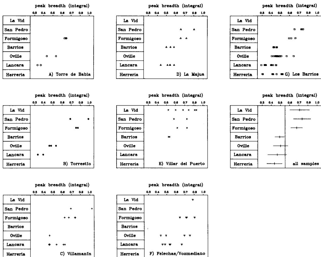
Fig. 6.—Dependence of the IC on the stratigraphic position at several localities in the Somiedo-Correcilla Unit. Everywhere, the jump from the anchizone (Cambro-Ordovician) to diagenesis (Siluro-Devonian) is obvious. Localities as in fig. 5. In the «all samples» diagram, means and their 99 % confidence levels are given.
