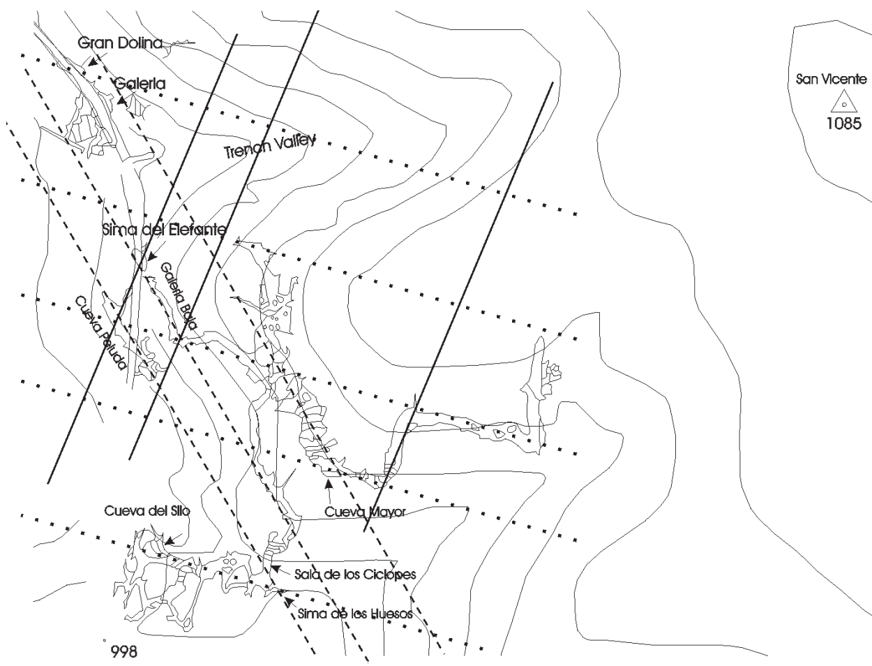
Fig. 7.—Plan of the Atapuerca karst system after G. E. Edelweiss (Martín Merino et al. , 1981). Superimposed on it, lines defining the planes measured on the Sima del Elefante limestone walls has been drawn. Also, several parallel lines to those planes has been recorded on the plan. Also, an extra set of parallel lines following the axis main galleries has been put on the plan. Structural features of the Sima del Elefante and its development may be initially understood in the context of the major structural features of the Atapuerca cave network. Note, for instance, that cave entrances are located at joint points of major structural planes; the TE site being an example of this pattern.
