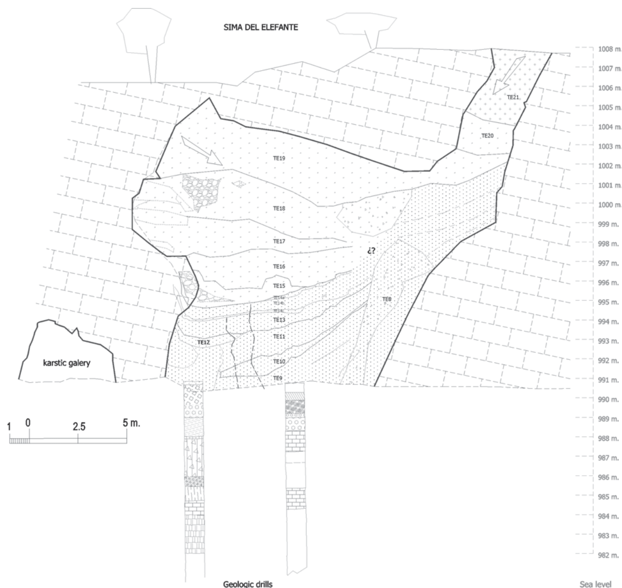
Fig. 2.—The topographic profile of the Sima del Elefante site (Atapuerca). Cave section at the level of railway-trench limestone cut. Main contact lines and stratigraphic units are indicated. At the bottom, below the present ground level, stratigraphic succession of non-exposed sediments coming from core samples. Scale indicates the heights on the sea level and the archaeological reference from the zero level chose for the excavation of the site.
