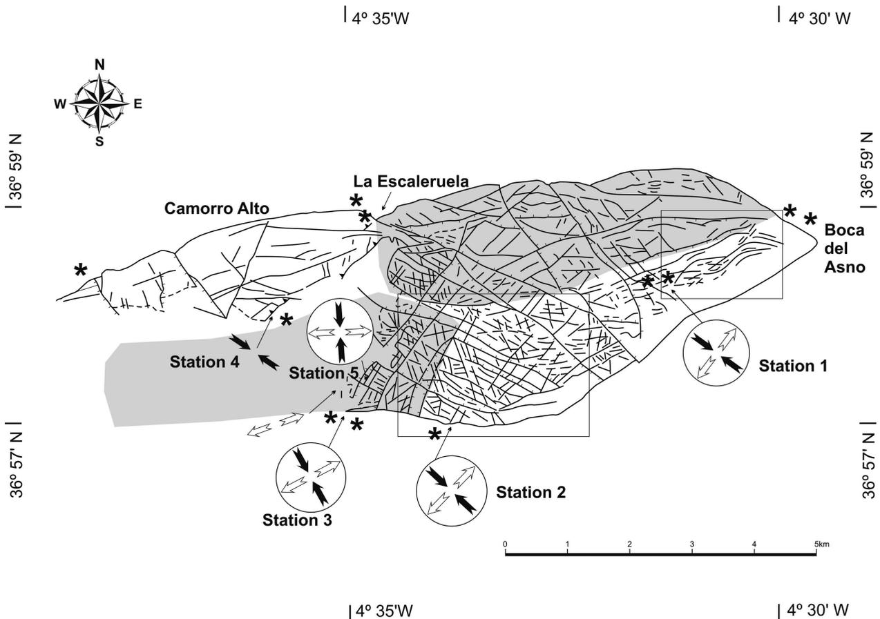
Figure 5.—Sketch of the fractures in the Torcal-Camorro Alto area. The position of the five stations of measures of minor structures (Fig. 7) is indicated. There, black arrows show the direction of compression, white arrows the direction of tension. Stars indicate other points where minor structures were measured. Grey colour differentiates the NE and SW sectors. The squares indicate the positions of D of the figure 3 and E of the figure 6.
