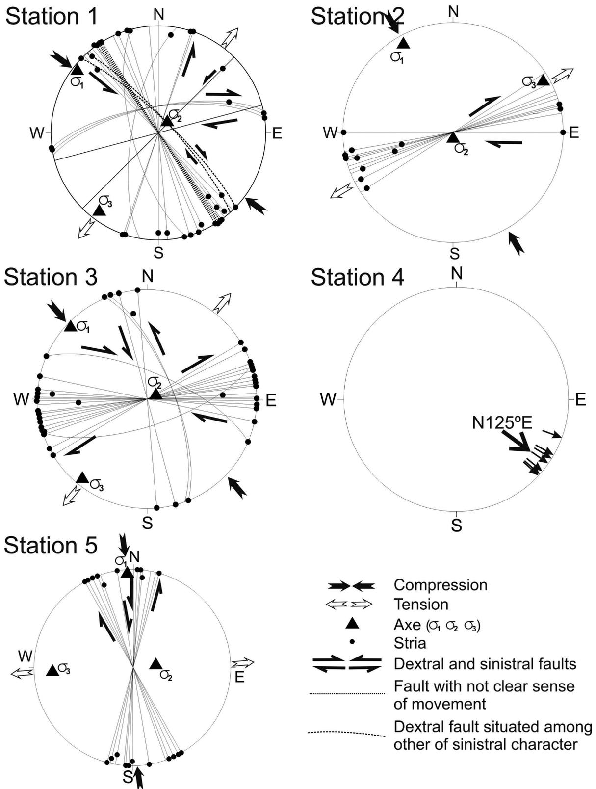
Figure 7.—Diagrams of the different stations of measures (equal area projection, lower hemisphere). Their position are indicated in Fig. 5.
