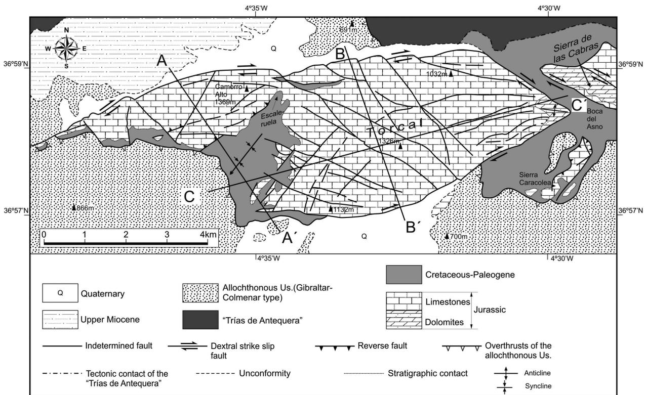
Figure 2.—Simplified geological map of the Torcal de Antequera. The positions of the cross-sections of Figure 4 are indicated. Its location is indicated in Figure 1.
