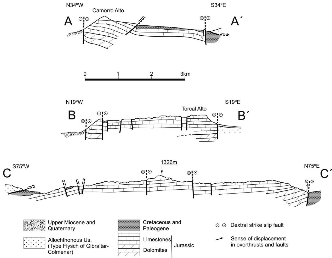
Figure 4.—Geologic cross-sections of the Torcal. Their positions are indicated in Figure 2.
